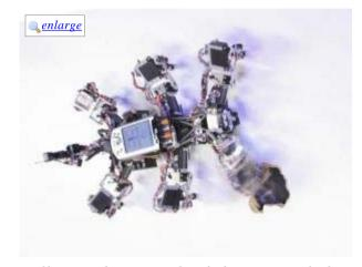
Following the principle of chaos control, the robot produces regular leg movements when walking normally. In addition, it can use the uncontrolled chaotic movement pattern to free itself when its leg is trapped in a hole. (Credit: Network Dynamics Group, Max Planck Institute for Dynamics and Self-Organization)
