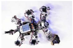
Chaos frees the robot from a trap An electric circuit consists of two simulated neurons generates the rhythm, after which the robot moves its six legs. Special feature: The neurons oscillate chaotically. © Network Dynamics Group, Max Planck Institute for Dynamics and Self -
