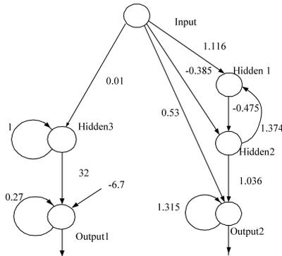
Fig. 7. The combined network recognizes low-frequency sound around 100 Hz (Output 1), and the tactile signal around 2000 Hz (Output 2).
