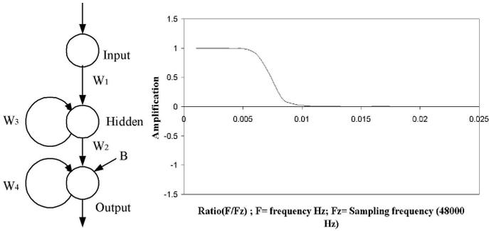
Fig. 4. Left: a simple and robust network for auditory processing, performing as a low-pass filter for noisy signals with varying amplitude. The bias term  $B$  is equal to  $-6.7$  and all weights are positive,  $W_1 = 0.01$ ,  $W_2 = 32$ ,  $W_3 = 1$  and  $W_4 = 0.27$ . Right: the characteristic curve of the network displaying the cut off frequency at 300 Hz.
