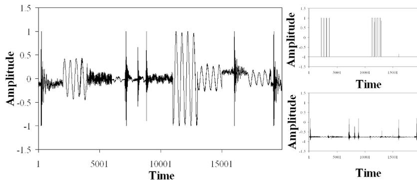
Fig. 10. Left: mixed input signals, sound at 100 Hz and tactile signals, for the network. Right: signals at output 1 (upper right) and 2 (lower right); they are active only for sound and tactile signals, respectively. All other signals are suppressed. All figures use the same scale in x- and y-axis.
