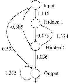
Fig. 6. A network processing tactile sensor signals. It filters the low-frequency sound. Its output signal follows the tactile signal, which has a high frequency around 2000 Hz.
