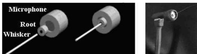
Fig. 1. The auditory-tactile sensor consisting of a whisker of a real mouse, a rubber root and a capacitor microphone. Left: assembly parts of a sensor; Right: the real sensor including a preamplifier circuit.
