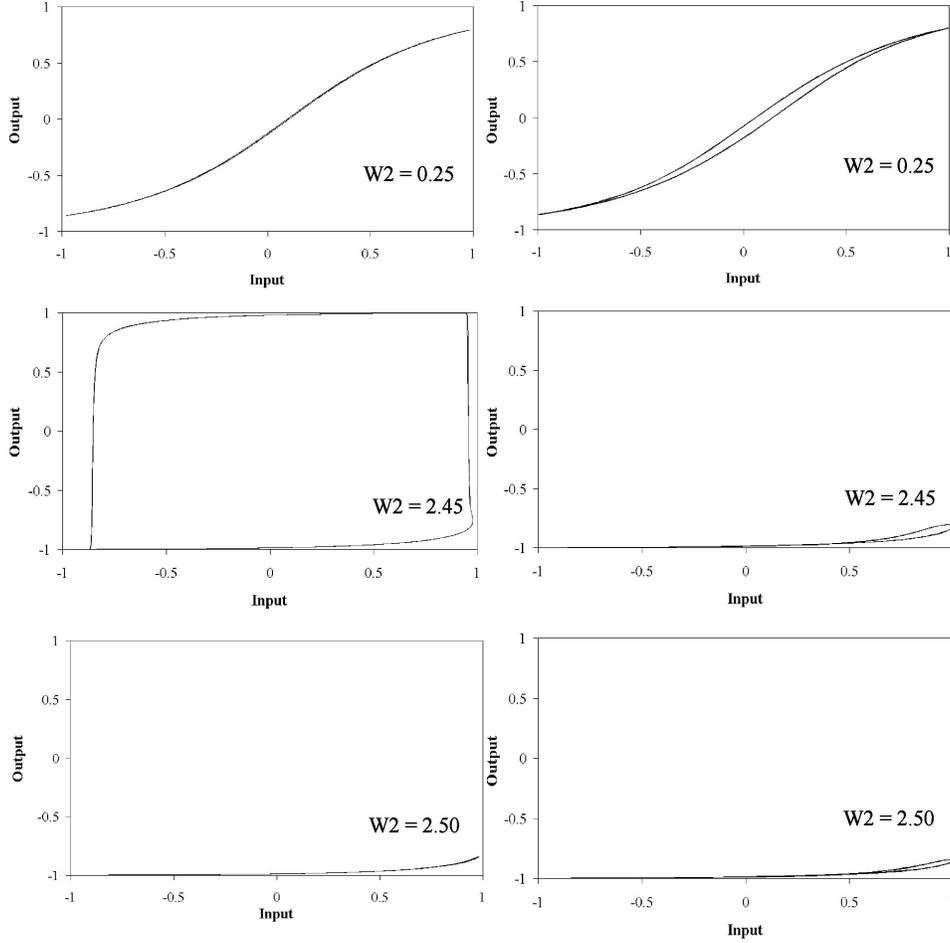
Fig. 3. Comparison of the “hysteresis effects” between input and output signals of high-and low-frequency sounds for  $W_2= 0.25, 2.45$  and  $2.50$ , respectively. Left: low-frequency sound (100 Hz); Right: high-frequency sound (1000 Hz).
