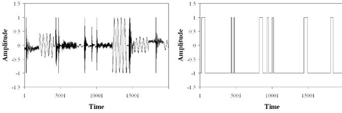
Fig. 5. Left: real signals coming from the physical sensor. Right: the corresponding target function.
