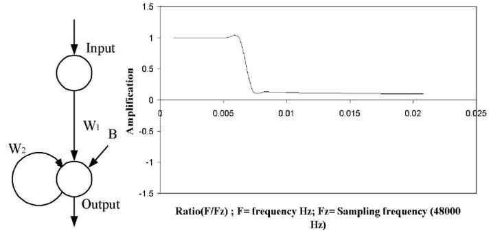
Fig. 2. Left: a simple network realizing a low-pass filter ; parameters are  $W_1 = 1$ ,  $W_2 = 2.45$  and  $B = -0.1$ . Right: the characteristic curve of this network with its cut off frequency at 300 Hz.
