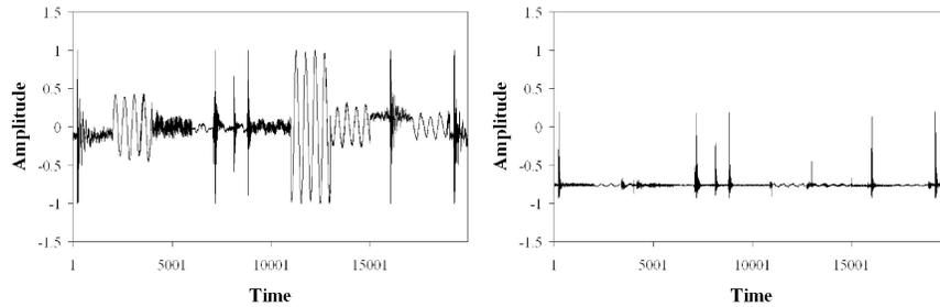
Fig. 9. Left: mixed input signals with sound at 100 Hz and the tactile signal. Right: the response of the network to the tactile signal. Both figures use the same scale in x-axis and y-axis.
