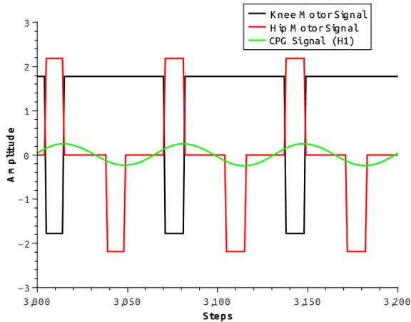
Fig. 4 Hips and knees motor signals generated by the CPG-based neural network.
