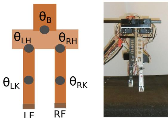
Fig. 1 Left: DACBOT schematic showing joints and feet.  $\theta$  refers to an active joint.  $LF, RF$  are left and right foot contact sensors. Right: Real DACBOT setup.
