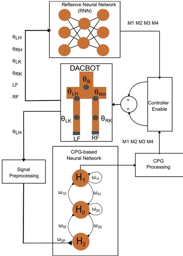
Fig. 2 The combination of the reflex-based or reflexive neural network ([10]) and the CPG-based neural network ([11]). They interact to drive the DACBOT system to achieve dynamic, robust, and adaptive locomotion. A controller enable is used to switch from reflex-based to CPG-based control and vice versa.  $\theta_{LH,RH,LK,RK}$  are left hip, right hip, left knee, and right knee joint angle feedback.  $LF, RF$  are left and right foot contact feedback.  $M_{1,2,3,4}$  are motor commands.
