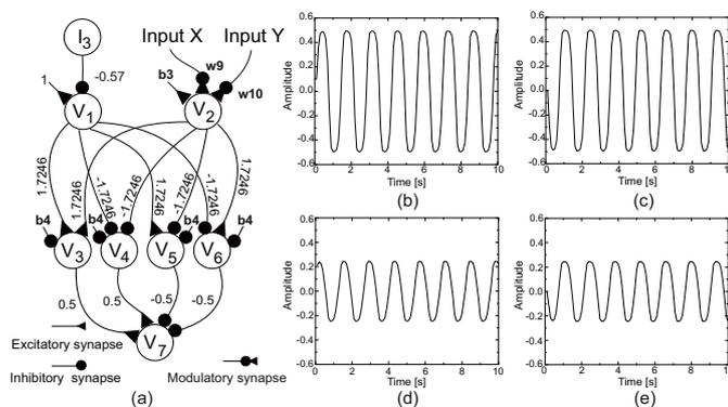
**Fig. 4.** (a) The velocity regulating network of the VRN1 module. The bias  $b_4$  is equal to -2.48285. The VRN2 module has the same structure. (b-e) Different output signals of the VRN1 module for forward/backward walking (b), hard pushing (c), soft pushing (d), boxing-like motion (e). The VRN2 output behaves in a similar way.
