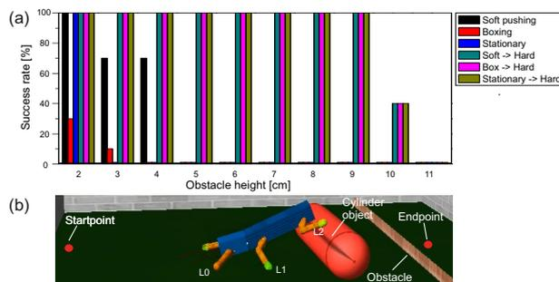
**Fig. 6.** Result of the obstacle test for the different object manipulation techniques. (a) Success rate in a total of ten experiments for each strategy. (b) The startpoint and endpoint locations from which the robot has to transport the object. In this experiment the robot was activated to walk backward without any additional steering command.
