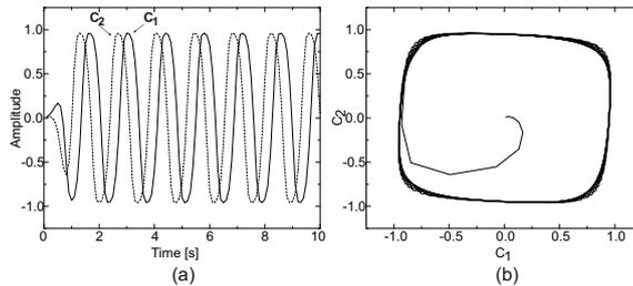
**Fig. 2.** (a) The periodic output signals from the CPG with the defined parameters shown in Fig. 1(a). Here we use the output signal  $C_1$  for generating locomotion and object manipulation. (b) The phase space with the quasi-periodic attractor of the oscillator network [17].
