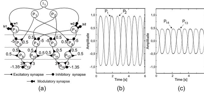
**Fig. 3.** (a) The phase switching network of the PSN1 module. The other PSN modules have the same structure. (b) The inputs of the PSN1 module which come from the CPG module. (c) The outputs of the PSN1 module where  $I_{1,2}$  are set to  $(1,1)$  or  $(0,1)$ . The outputs are inverted if  $I_{1,2}$  are set to  $(1,-1)$ ,  $(-1,-1)$ , or  $(1,0)$ . Note that the inputs and outputs of the other PSN modules behave in a similar way.
