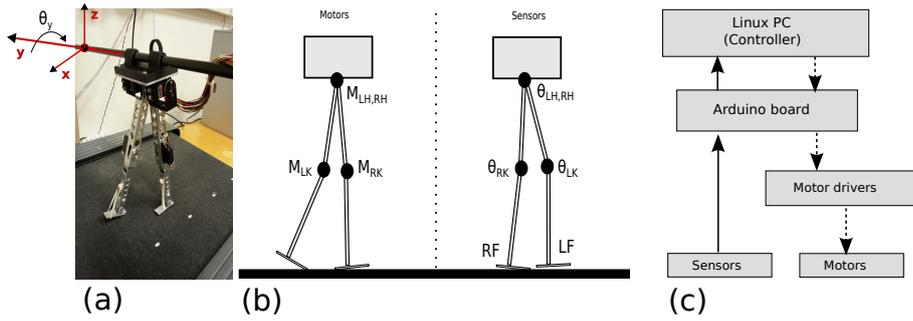
**Fig. 4.** (a) The planar bipedal robot DACBOT. For our experiments here, we constrain the robot such that it can only rotate along the y-axis. (b) Motors and sensors of DACBOT. (c) Schematic of the DACBOT setup.
