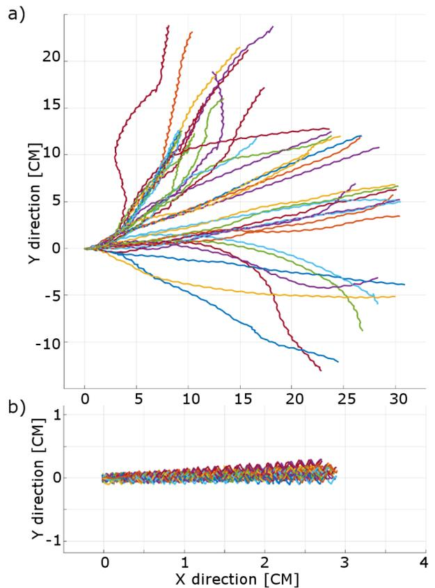
Fig. 4 a) The walking experiments show robot trajectories for 45 runs within about 120 seconds for each run. b) The ball rolling experiments show robot trajectories for 50 runs within about 110 seconds for each run.
