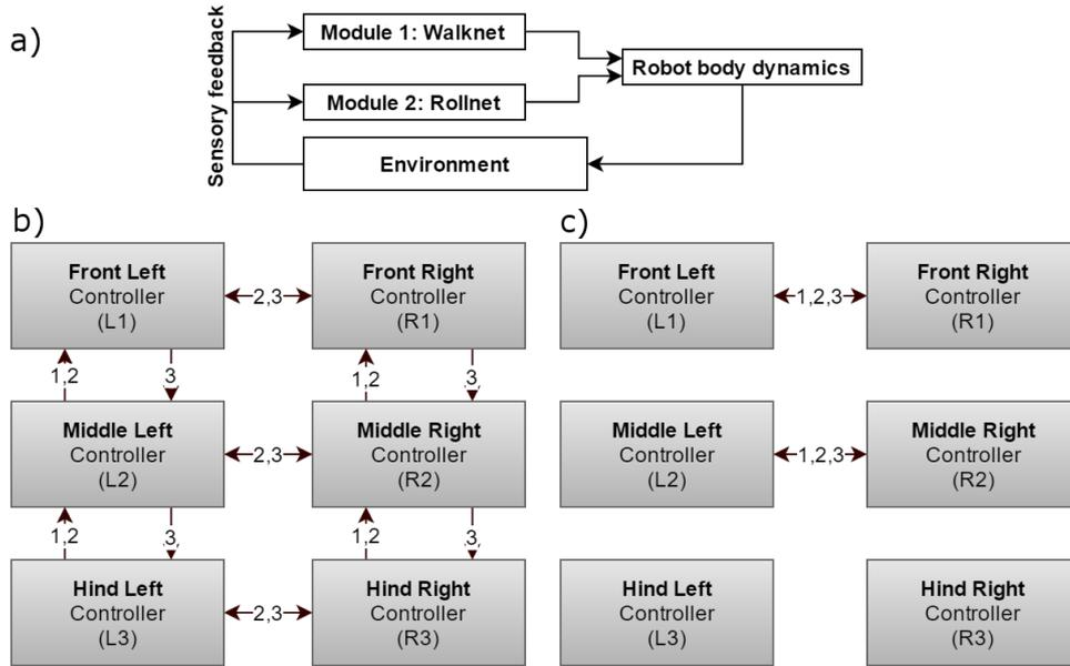
Fig. 2 a) Distributed sensor-driven control of a dung beetle-like robot. It consists of two subnetworks or modules: Walknet for walking and Rollnet for ball rolling. b) The influences of the Walknet rules on the legs for walking. c) The influences of the Rollnet rules on the legs for rolling a ball.
