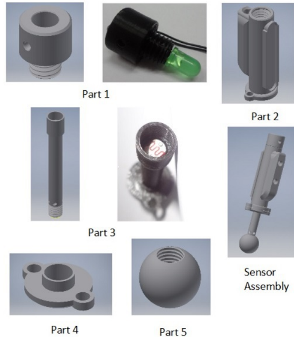
Fig. 2 All parts were 3D printed. Part 1 and part 3 are shown in both the CAD model and 3D print.
