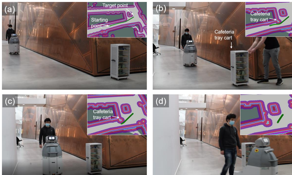
Supplementary Figure 1. SMOOTH robot successfully guiding a subject in a dynamic environment (situation 1). (a) It guided the subject from the starting point towards the target point. (b) A cafeteria tray cart was moved to block the planned path. The robot detected the cart and reactively adjusted its path to avoid the cart. (c) It successfully avoided the cart. (d) It continued to guide the subject to the target point. The experimental video of this experiment can be seen at http://www.manoonpong.com/ProactiveControl/video5.mp4 . The light condition during this experiment was approx. 250 lux. The inset of each snapshot shows the navigation map and trajectory (green line) of the robot.
