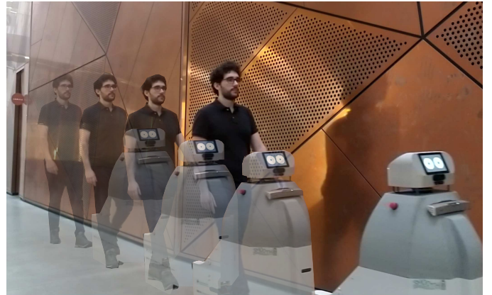
Fig. 1. Example of the SMOOTH robot with proactive control for online individual user adaptation in a guidance scenario. The robot navigates and guides the user in the relevant environment (e.g., inside a build at the University of Southern Denmark (SDU)). The proactive robot system has been successfully demonstrated to support elderly people in an operational environment (i.e., the Ølby elderly care center in Køge, Denmark).
