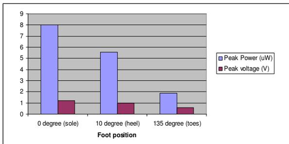
Figure 12: Peak voltage and peak power at prosthesis foot positions
