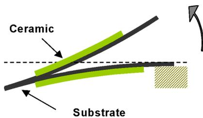
Figure 2: Diagram of the PZT piezoelectric
